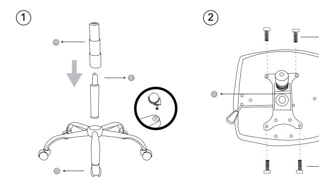
Push and twist the wheels into the star base. And place the cylinder cover over the gas lift. Align the butterfly mechanism with the screw holes at the bootom of the seat as shown in image above.
