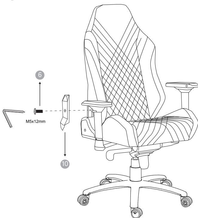
Fasten the backrest with provided screws.
