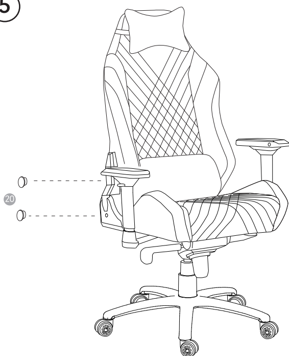
Fasten the side covers, and put the small side cover on
